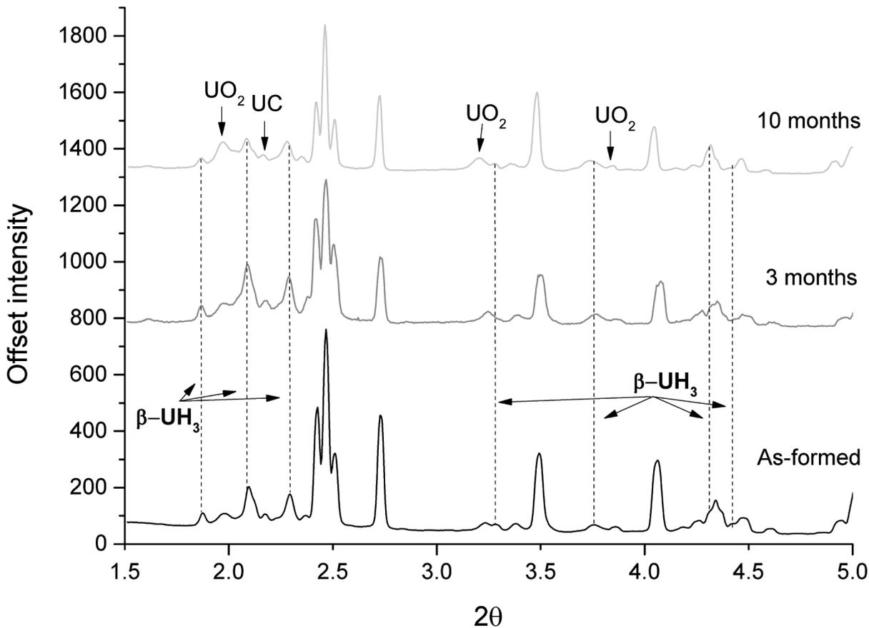
**Fig 1. XRPD results of hydrided uranium, encapsulated in cement after 0, 3 and 10 month submersion in de-ionised water.** The data was normalised to the first UO<sub>2</sub> peak, as this was considered the least strained constituent of the sample. Intensities of peaks at each time period vary due to imperfect beam line set up at each occasion. All unlabelled peaks are ascribed to uranium.
