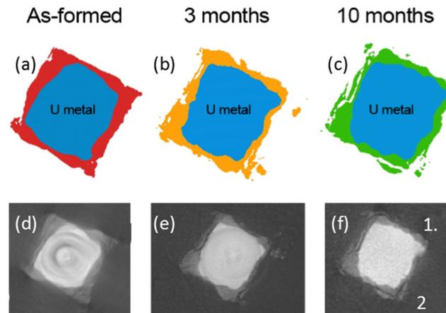
**Fig 3. Cross sections at the same position of the uranium encapsulated in grout over time.** Images (a) to (c) are accurate representations of the uranium (blue) and surrounding corrosion products (red, orange and green) perpendicular to the length of the sample. Images (d) to (f) are radiographs corresponding to the above representations, but with the additional surrounding grout.
