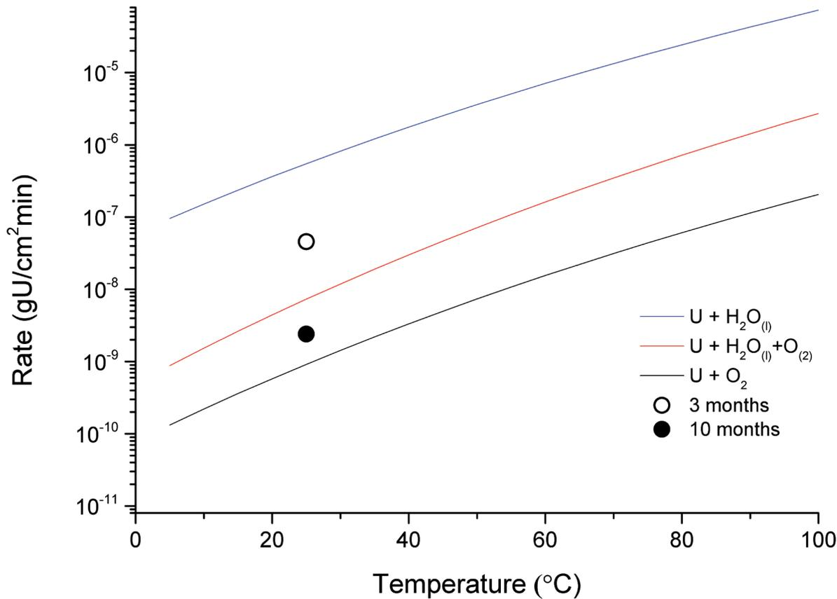
**Fig 4. A comparison of the measured oxidation rates (R) to the empirically derived models for the  $U + 2H_2O_{(l)} \rightarrow UO_2 + 2H_2$ ,  $U + 2H_2O_{(l)} + O_{2(g)} \rightarrow UO_2 + 2H_2O$  and  $U + O_{2(g)} \rightarrow UO_2$  systems provided by Delegard and Schmidt, Ritchie and Haschke respectively [5,12,19]. Results collected from the initial investigation [13] are also presented; Bare U (i.e. no grout) and U + grout (i.e. after 1 week encapsulated in grout).**
