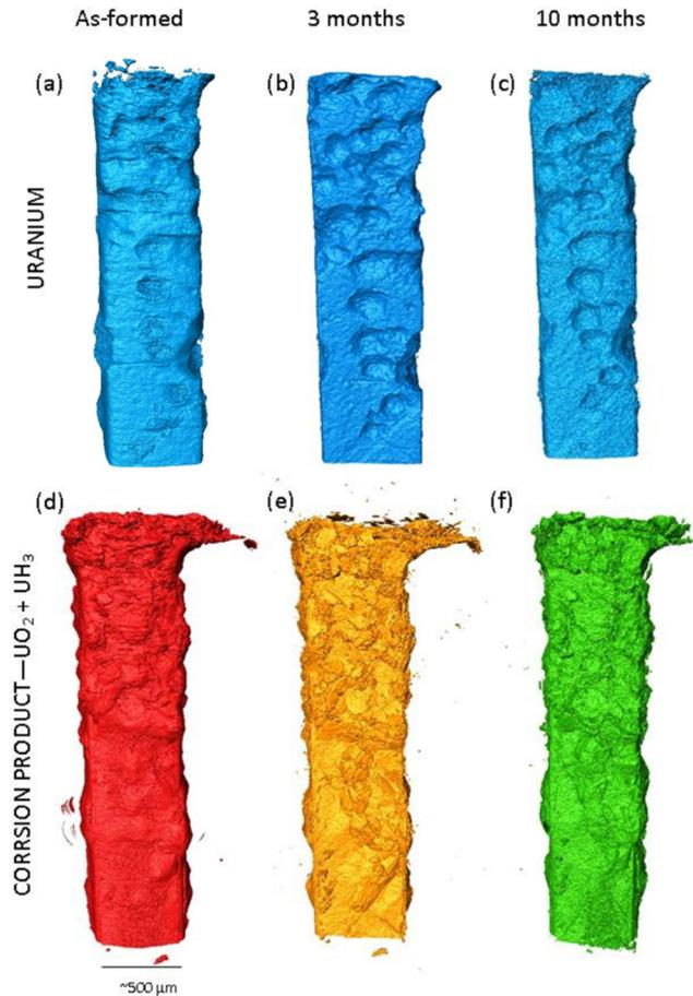
**Fig 2. Three dimensional representations of the uranium sample encapsulated in cement over the 10 month period.** Images (a) to (c) display what is left of the uranium inner core after initial hydriding (a) to 10 month submersion in water (c). Images (d) to (f) show the corresponding corrosion layers associated with each time period (0 to 10 months).
