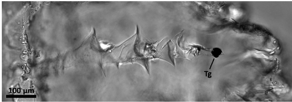
Fig. 3. A keystone with a NWA 10256 CR2 chondrite magnetite terminal grain, shot into aerogel at 6.10 \text{ km s}^{-1} using the light-gas gun at the University of Kent (Burchell et al. 2008). The remaining track stylus cut from the aerogel, minus the bulbous region, measures 650 \text{ }\mu\text{m} with a \sim 30 \text{ }\mu\text{m} terminal grain.
