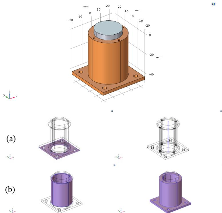
**Figure 5.** Copper and silicon interference fit model with a 60  $\mu\text{m}$  gap at room temperature.
