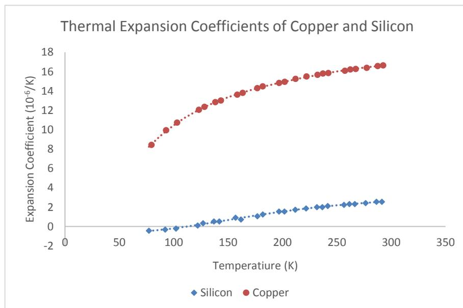
**Figure 3.** Thermal expansion coefficients of Silicon and Copper.
