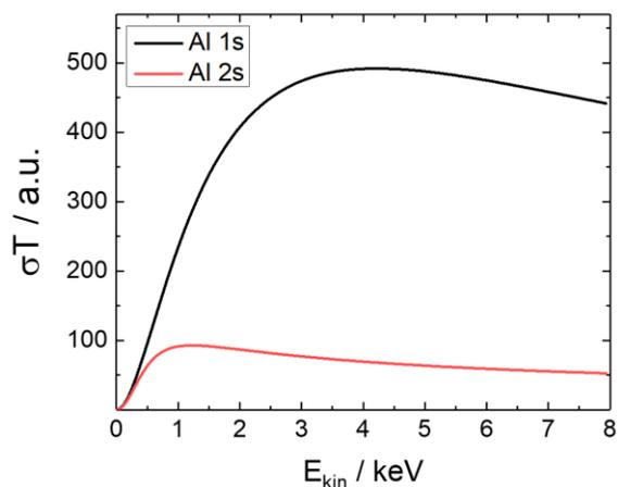
Figure 10. The product of the photoionization cross-section  $\sigma$  and measured transmission  $T$  for 15 nm membrane as a function of kinetic energy for Al 1s ( $E_b = 1559.6$  eV) and Al 2s ( $E_b = 117.8$  eV) core levels;  $\sigma T$  is proportional to the electron yield through the membrane. The photoionization cross section  $\sigma$  is taken from Scofield [1] for the corresponding X-ray excitation energy  $E_\gamma$  and subshell.
