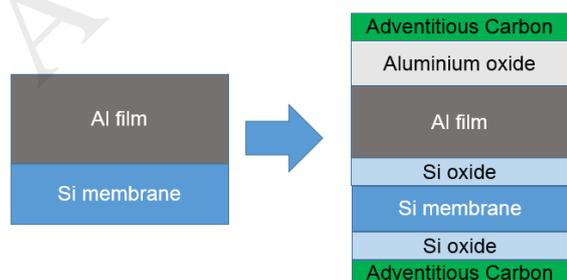
Figure 7. The ideal sample (left) and the real sample (right)
