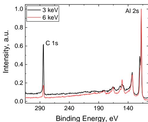
Figure 6: Spectra obtained with 3 keV and 6 keV excitation energy showing carbon contaminations on the aluminium film.
