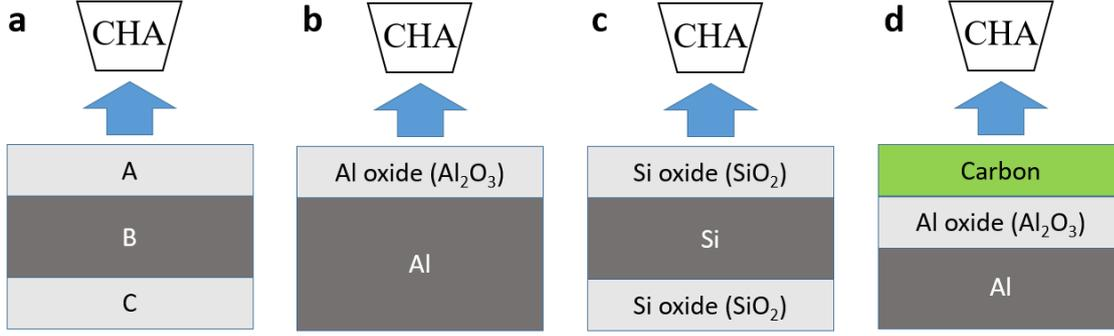
Figure 8. (a) photoelectrons emitted from a generic three layer structure to the photoelectron analyzer (CHA), (b) emission from a two layer structure to estimate the thickness of Al oxide, (c) a three layer structure to estimate Si oxide thickness and (d) a three layer structure to estimate the thickness of carbon layers.  $\text{Al}_2\text{O}_3$  is present only on top of the Al film and carbon present only on both outer faces
