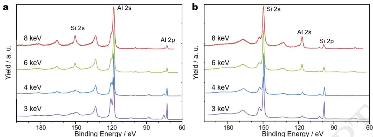
Figure 2. Photoelectron spectra of the Al 2s region measured at 3, 4, 6 and 8 keV excitation energy for the sample with 15 nm Si membrane shown on a linear scale with (a) the Al film facing the analyzer and (b) the Si membrane facing the analyzer (cf. Fig. 1). The spectra recorded for 4, 6 and 8 keV are vertically offset for clarity. All spectra in (a) and (b) are normalized to the Al 2s and Si 2s peaks, respectively and shown on a linear scale.
