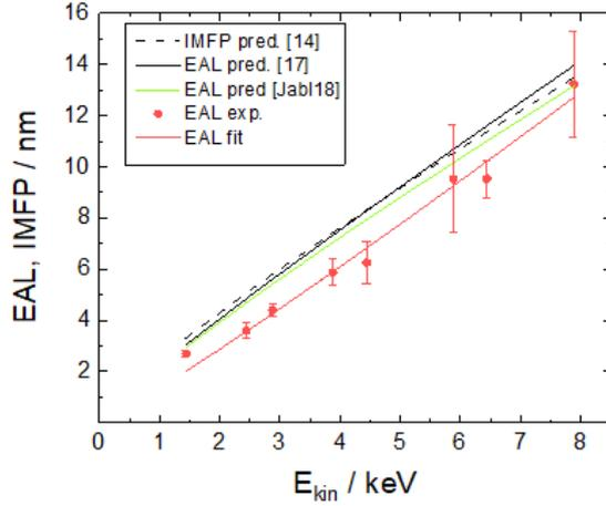
Figure 9. Experimentally determined effective attenuation length in silicon (experimental values - red points, power law fit - red solid line). For comparison effective attenuation length from [20] (black solid), from [21] (green solid) and inelastic mean free path (black dashed) from [4] are shown.
