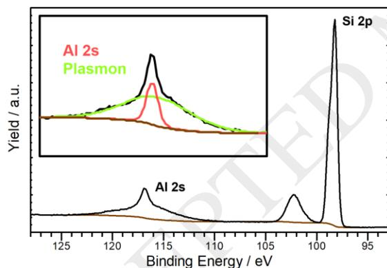
Figure 3. Al 2s peak and the neighbouring Si 2p at  $E_\gamma = 3$  keV for membrane to analyzer geometry. The inset shows a close up view of Al 2s region with a fit of Al 2s elastic peak (red) and Si plasmon of Si 2p (green).
