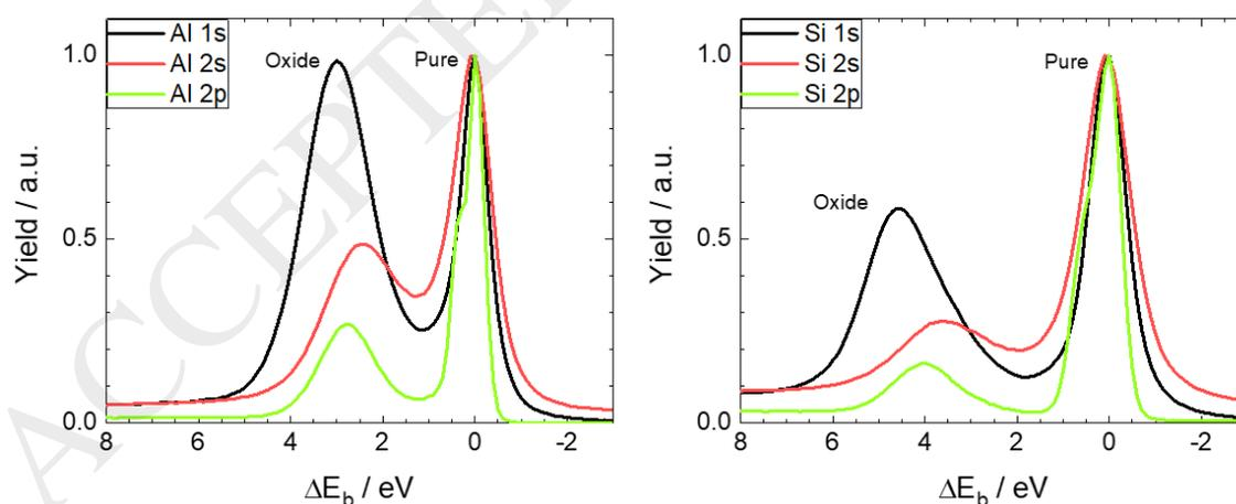
Figure 5. Al (left) and Si (right) 1s, 2s and 2p core levels for 3 keV excitation energy showing the intrinsic peak and a strong higher binding energy component due to oxidation. All spectra are normalized to the intrinsic (pure) peak.
