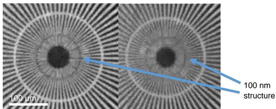
Figure 4: Comparison of TXM operation using different bandpass of the monochromator's multilayer systems. Left: Mo-B<sub>4</sub>C strip with 1% bandwidth, right Ru-B<sub>4</sub>C with 5% bandwidth. 100 nm structures are visible on the left image.
