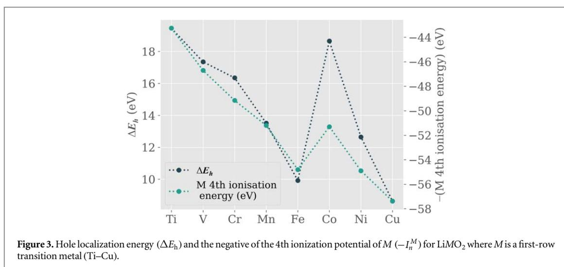
**Figure 3.** Hole localization energy ( $\Delta E_h$ ) and the negative of the 4th ionization potential of  $M$  ( $-I_n^M$ ) for  $\text{LiMO}_2$  where  $M$  is a first-row transition metal (Ti–Cu).
