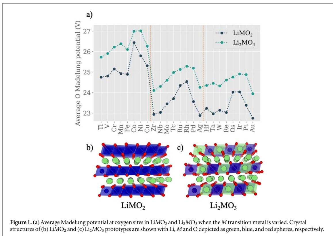
**Figure 1.** (a) Average Madelung potential at oxygen sites in  $\text{LiMO}_2$  and  $\text{Li}_2\text{MO}_3$  when the  $M$  transition metal is varied. Crystal structures of (b)  $\text{LiMO}_2$  and (c)  $\text{Li}_2\text{MO}_3$  prototypes are shown with Li,  $M$  and O depicted as green, blue, and red spheres, respectively.
