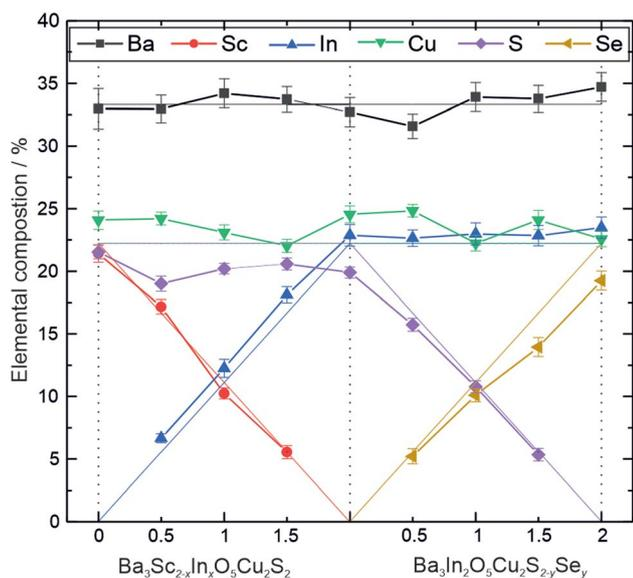
**Fig. 2** Plot of elemental composition as determined by EDX excluding oxygen, for the two solid solutions:  $\text{Ba}_3\text{Sc}_{2-x}\text{In}_x\text{O}_5\text{Cu}_2\text{S}_2$  and  $\text{Ba}_3\text{In}_2\text{O}_5\text{Cu}_2\text{S}_{2-y}\text{Se}_y$ . Thin solid lines represent the percentage of each element expected based on the target composition.
