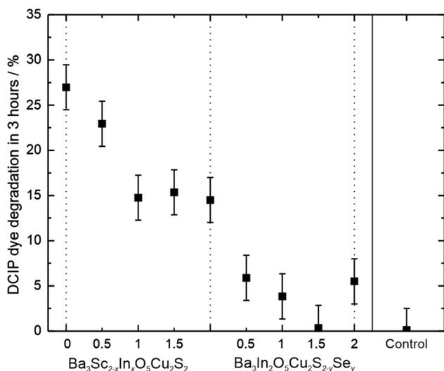
**Fig. 6** Plot of fraction of DCIP dye degraded after 3 hours exposure to a solar simulator in the presence of a sample of each of the oxychalcogenide powders, and a control with no sample present.
