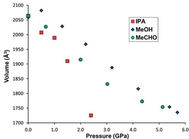
Fig. 4 Unit cell volume of STAM-1 in IPA (red squares), acetaldehyde (MeCHO) (green circles) and STAM-1<sub>MeOH</sub> in methanol (blue diamonds) and as a function of pressure.
