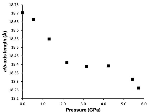
Fig. 5 Unit cell *a/b*-axes length of STAM-1<sub>MeOH</sub> in methanol as a function of pressure.
